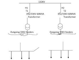
Fig. 2: One line schematic diagram of newly constructed 132/33kv sub-station along Abeokuta – Sagamu Express Road
